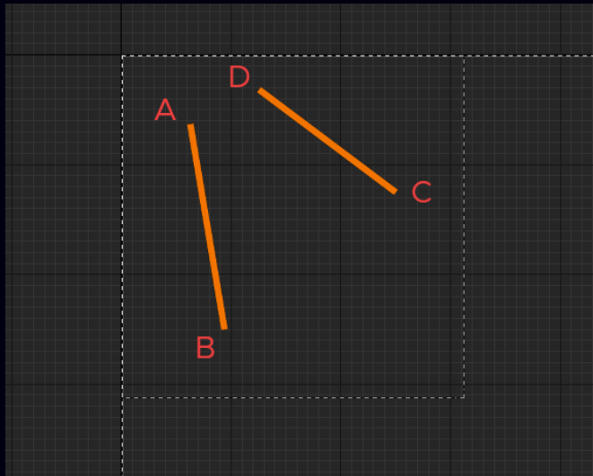
A Point Cloud drawn as lines connecting points A (100, 100) and B (150, 400); C (400, 200) and D (200, 50).
