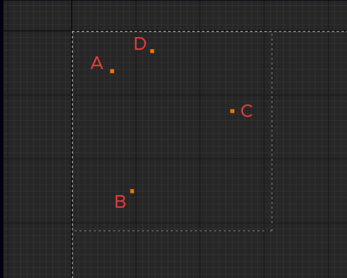
A Point Cloud drawn as separated points A (100, 100), B (150, 400), C (400, 200), and D (200, 50).
