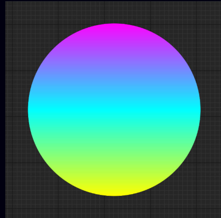
A Linear Gradient with Start Point (0.0, 0.0), End Point (0.0, 1.0), and three Stops.
